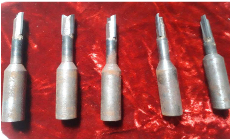
Figure 2. Five varieties of customized carbide tipped tools.
